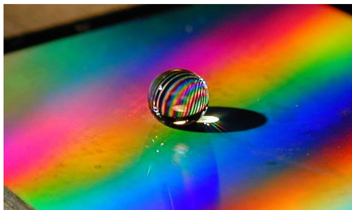
FIG. 1. An object of science. A water droplet placed on a textured, hydrophobic surface adopts the shape of a pearl. The texture is micrometric but its regularity makes it “visible,” owing to the structural colours it generates on the solid surface. (Photo: Mathilde Reyssat.)
