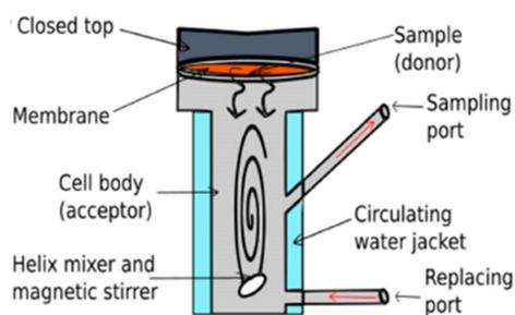
**Figure 5.** Franz-diffusion cell schematics (adapted with permission from Scientia Pharmaceutica, a MDPI Open Access Journal [119]).
