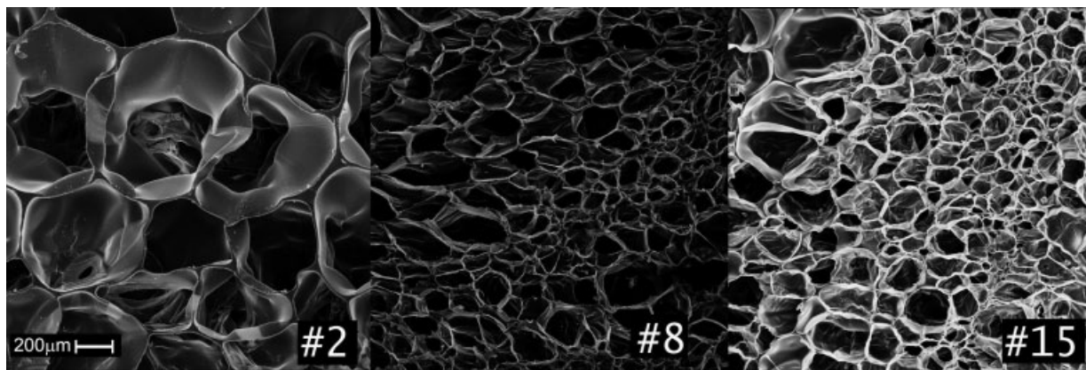
FIG. 5. SEM analysis of PCL batch-foamed with CO 2 , effect of the pressure drop rate (refer to Table 1 for numbering).
