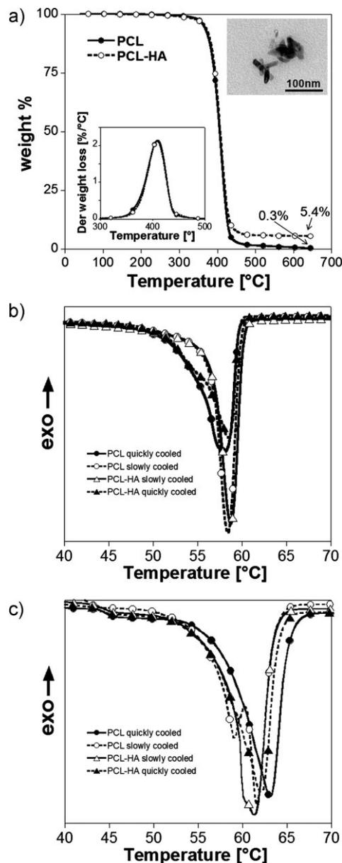
**Figure 1.** (a) TGA/DTGA results for neat PCL and PCL-HA nanocomposite; DSC 1<sup>st</sup> heating scan (2 °C min<sup>-1</sup>) of PCL and PCL-HA nanocomposite prepared by the slow and quick non-isothermal cooling processes before (b) and after (c) the scCO<sub>2</sub> treatment.
