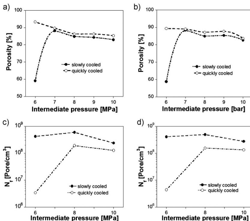
Figure 3. Porosity (a and b) and pore density (c and d) of the (a,c) PCL and (b,d) PCL-HA nanocomposite scaffolds as a function of the intermediate pressure and thermal history.
