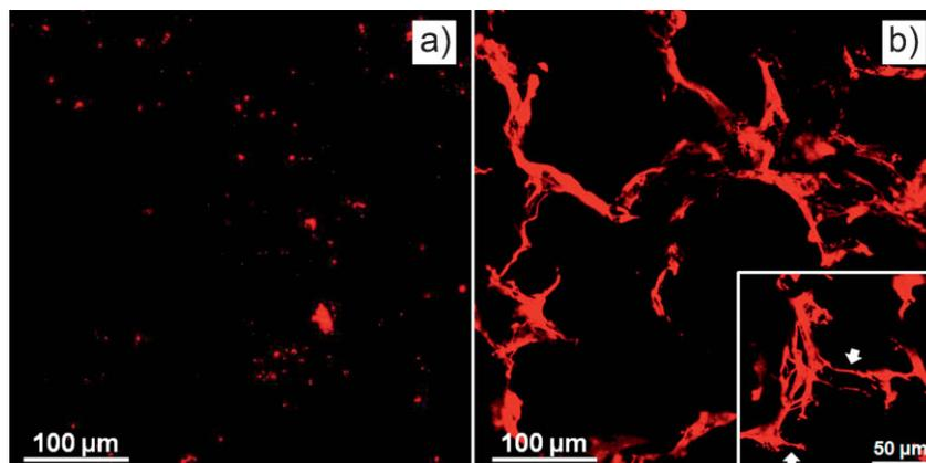
**Figure 4.** (a) CLSM image of a bimodal PCL scaffold without cells after 24 h of incubation in vitro; (b) CLSM image of the hMSCs seeded onto the bimodal PCL scaffold after 24 h of incubation in vitro.
