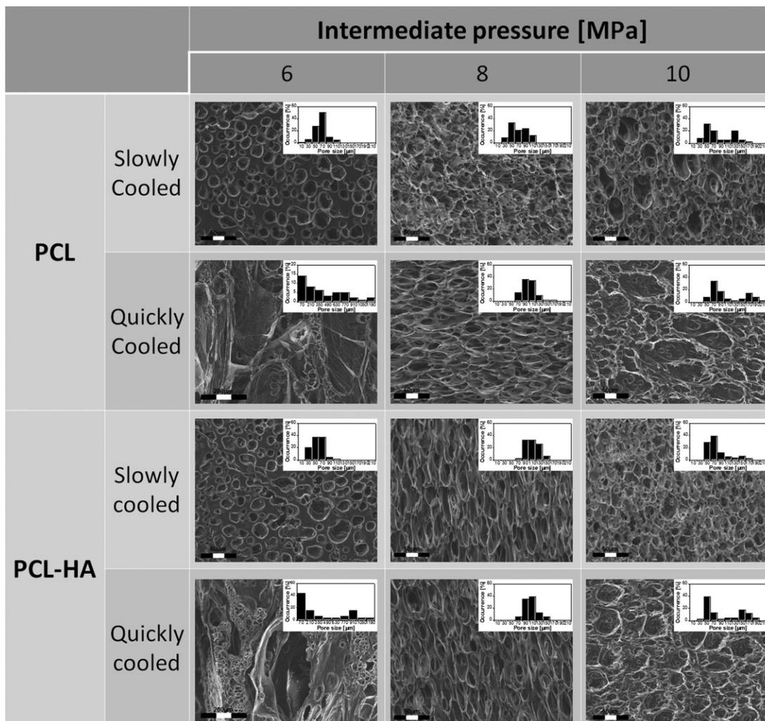
**Figure 2.** Morphology and pore size distribution of the PCL and PCL-HA nanocomposite scaffolds as a function of the intermediate pressure and thermal history.
