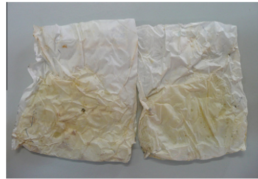
Fig. 3. Evidence of opacification and embrittlement of HP sterilized PLA film. Photograph of a PLA Biophan 121 film after HP sterilization of a pouches containing solid carrots as packaged foodstuff.
