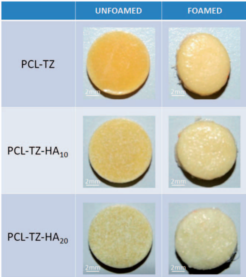
Figure 2. Macroscopic views of the multi-phase biomaterials before and after the gas foaming step.
