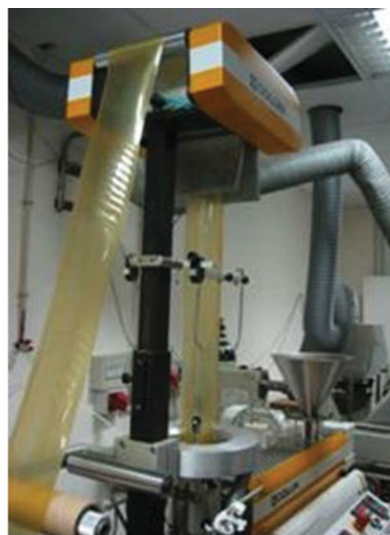
Figure 10 Picture of lab-scale film blowing of TPZe (batch A). [Color figure can be viewed in the online issue, which is available at www.interscience.wiley.com .]
