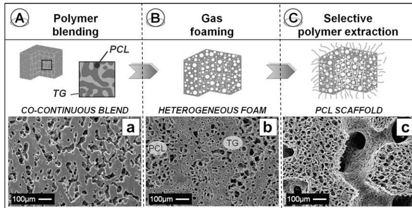
Fig. 1. Correspondence between the processing step and the microstructural evolution of PCL/TG system: (a) SEM micrograph of 3/2 (w/w) PCL/TG co-continuous blend after the selective extraction of the TG; (b) SEM micrograph of PCL/TG blend foamed with 4/1 (v/v)  $N_2/CO_2$  blowing mixture, at  $T_F = 44^\circ C$  and  $PDR = 700$  bar/s; (c) SEM micrograph of  $\mu$ -bimodal PCL scaffold prepared by the selective extraction of the TG from the foamed PCL/TG blend.
