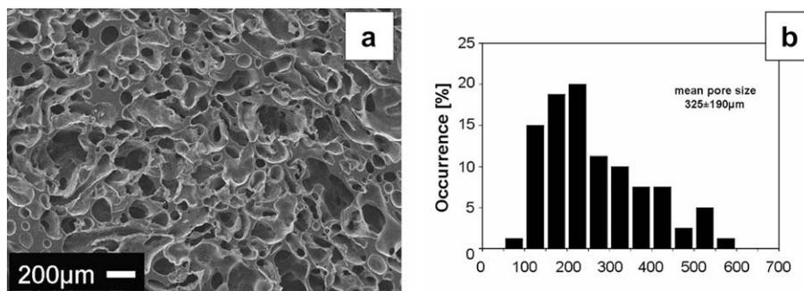
Fig. 7. (a) SEM micrograph and (b) pore size distribution of PCL scaffold with monomodal porosity distribution obtained by the GF/PE combined technology and performing the foaming process at  $T_F = 70^\circ\text{C}$ .
